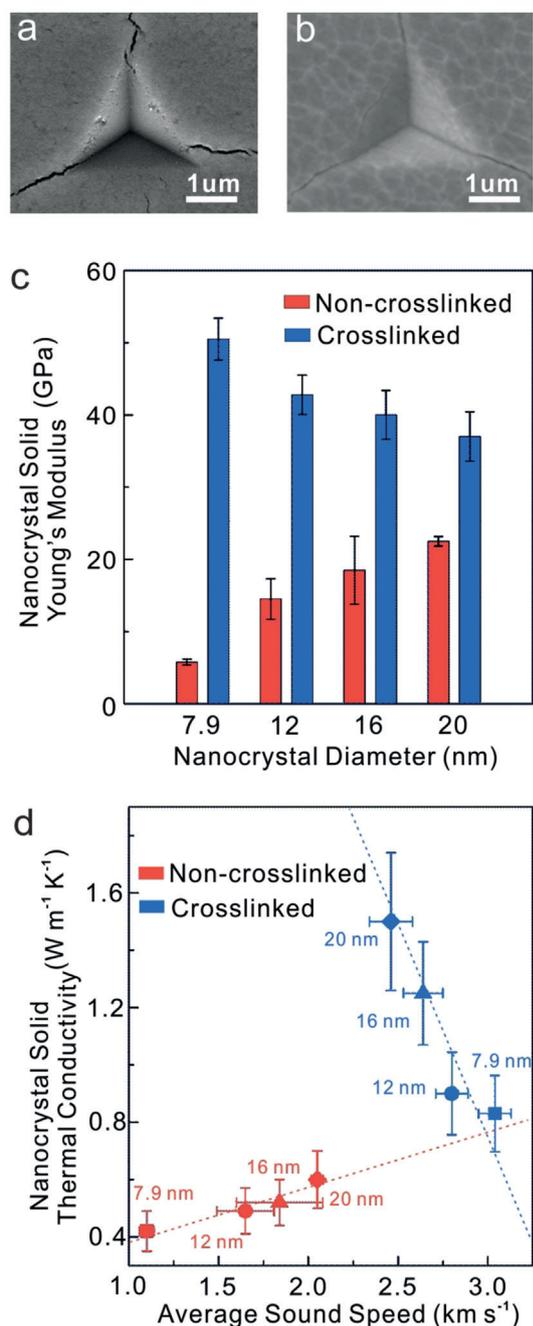
**Figure 4.** Representative SEM images of nanoindented iron oxide NC solids a) before and b) after annealing. c) Young's modulus of non-crosslinked and crosslinked iron oxide NC solids with varying NC core diameter. d) Thermal conductivity of non-crosslinked and crosslinked iron oxide NC solids as a function of derived average sound speed and varying NC core diameter.
